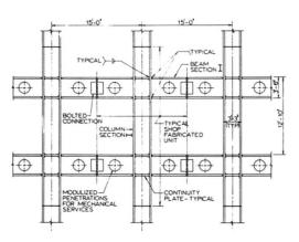
Fig. 5 Prefabricated beam - Column modules
