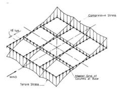
Fig. 4 Stress distribution due to wind load
