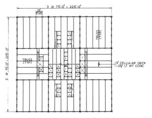
Fig. 2 Typical framing plan (levels 1 to 50) -Sears Tower
