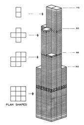
Fig. 3 Modular floor configuration — Sears Tower
