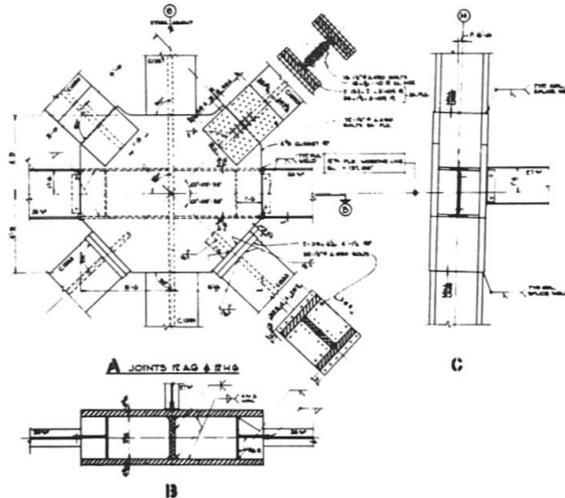
Fig. 4 Joint detail at 12th floor level
