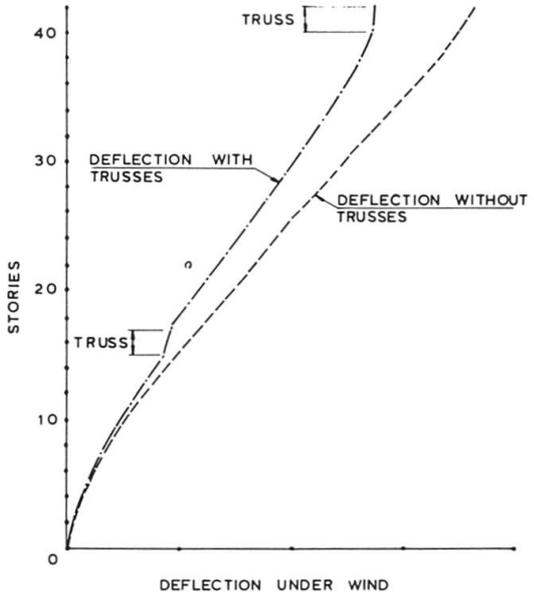
Fig. 4b Effectiveness of trusses in lateral resistance
