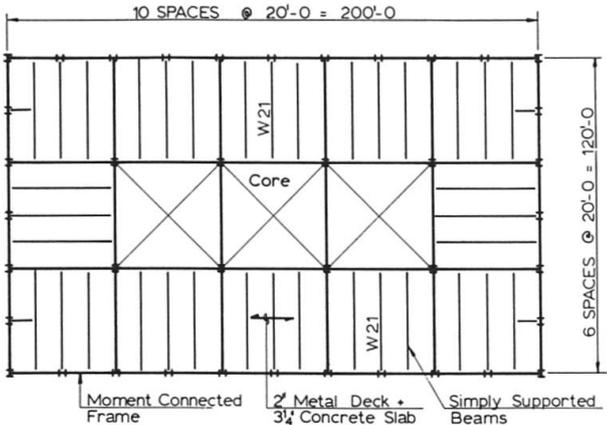
Fig. 2 Typical floor framing plan – First Wisconsin Center
