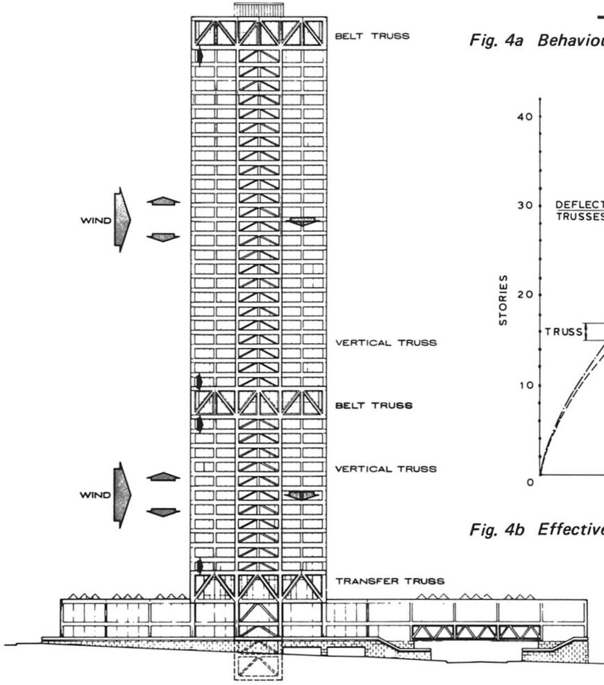
Fig. 3 East-West section showing lateral load resisting trusses
