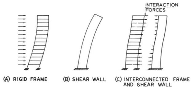
Fig. 3 Frame-shearwall interaction
