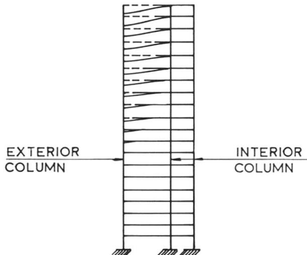
Fig. 4 Racking of floors due to temperature effect
