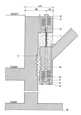
Fig. 3. Detail of final shell connection to tower shaft
