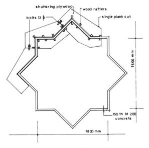
Fig. 1. Plan, shuttering details of shaft
