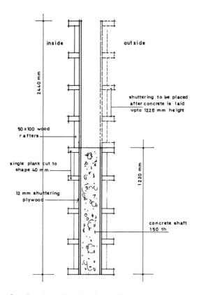
Fig. 3. Section, details of climbing formwork
