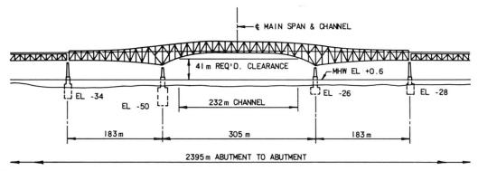
Fig. 1 Elevation main span. North and south bridges
