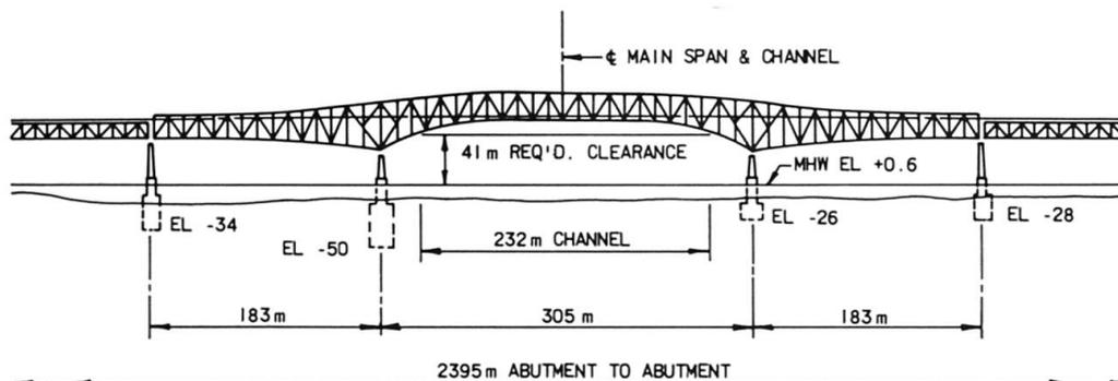
Fig. 1 Elevation main span. North and south bridges
