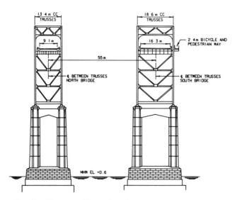
Fig. 2 Cross section of main spans
