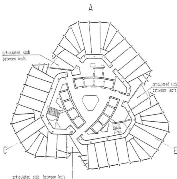
Fig. 1 Horizontal section through tower
