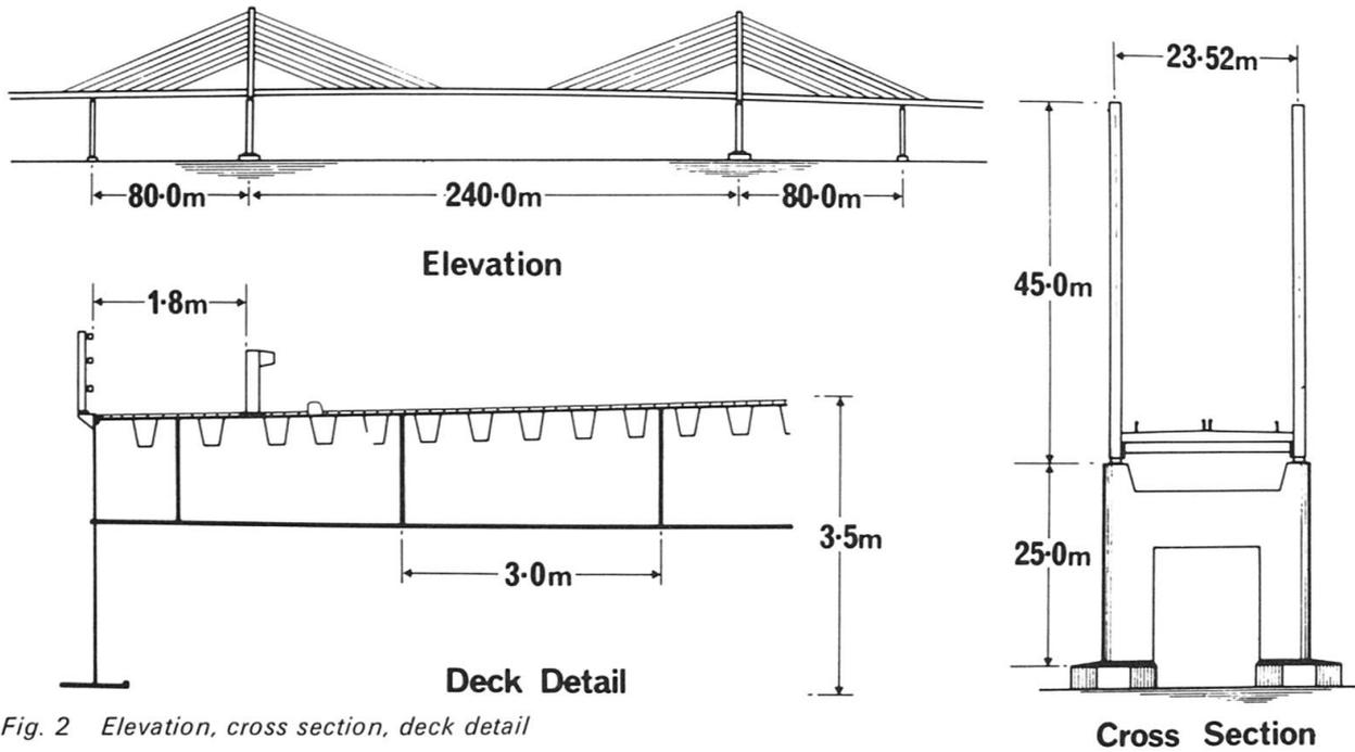
Fig. 2 Elevation, cross section, deck detail
