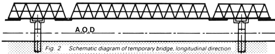
Fig. 2 Schematic diagram of temporary bridge, longitudinal direction
