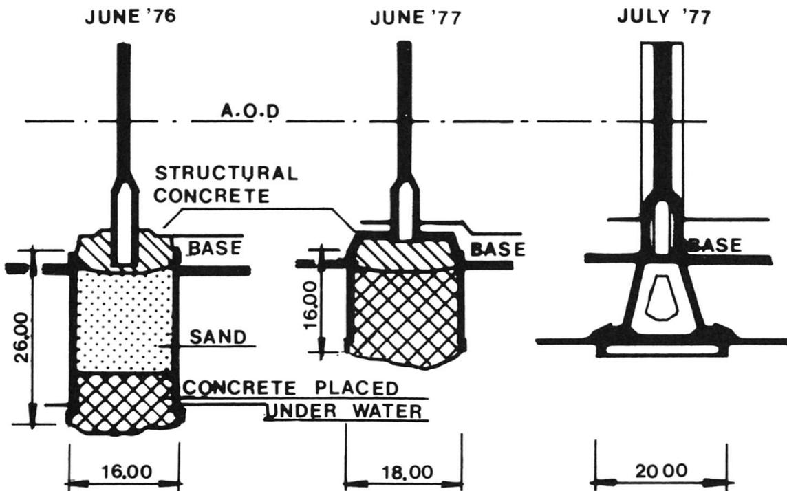
Fig. 7 Evolution of the design of the foundation
