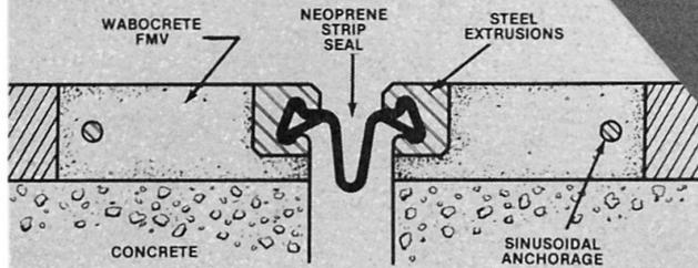
WABOCRETE FMV is ideal for lane-at-a-time rehabilitation work. Its rapid installation and heat fusion vulcanizing require about 2 hours. It serves as an energy absorbing, spall & crackfree, impervious expansion joint end dam in one piece from curb to curb.
