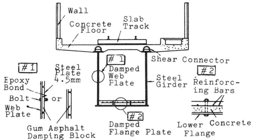
Fig. 4 Noise-control device for a composite bridge
