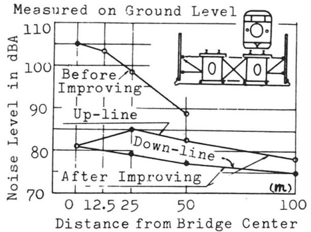
Fig. 2 Relation between noise-level and distance from bridge
