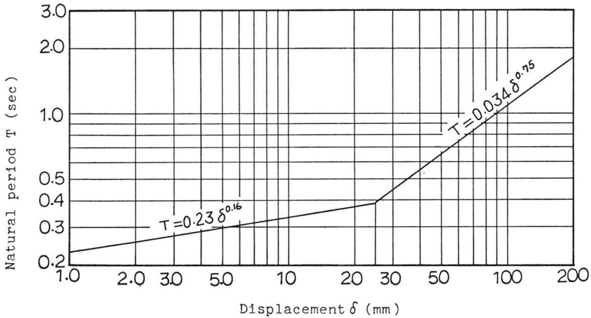
Fig. 2 Relation between natural period and displacement
