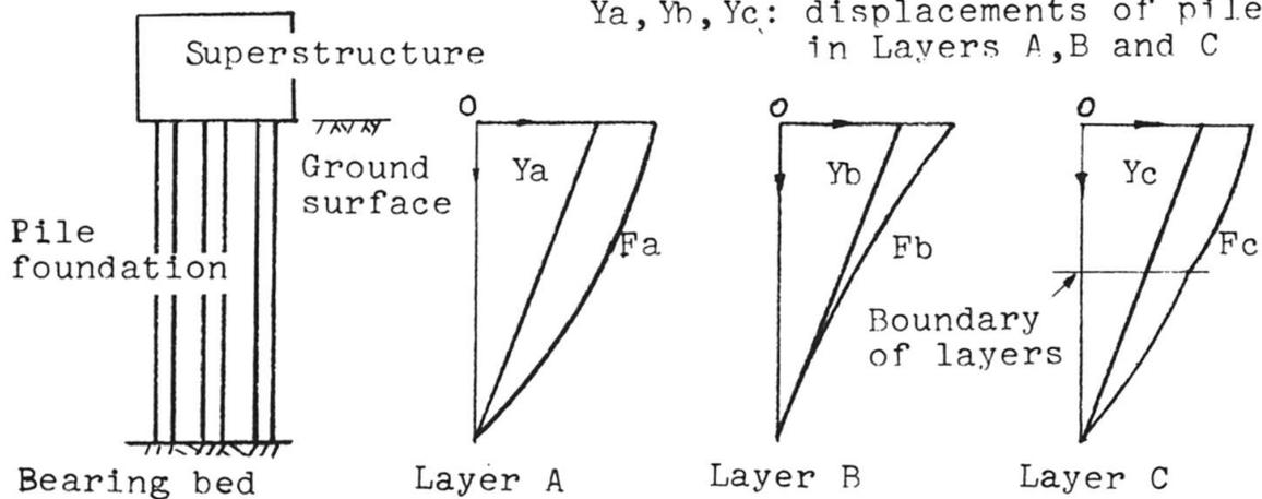
Fig. 3 Deformation patterns of grounds and piles
