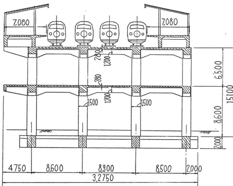
Fig. 1 Shinshirakawa station of reinforced concrete structure
