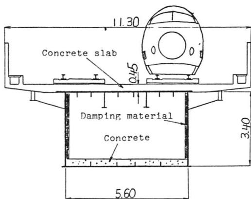
Fig. 6 Cross section
