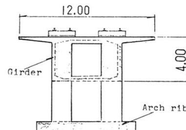
Fig. 8 Cross section (A-A)
