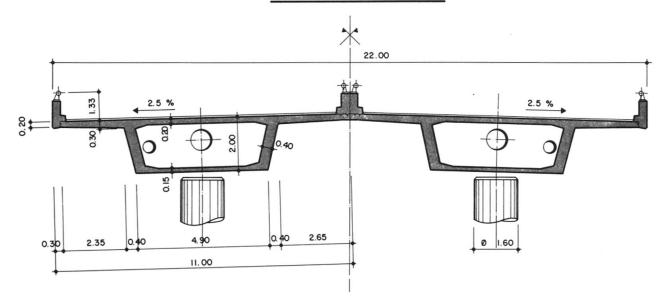
At its widest point, the cross-section of the superstructure is transformed into a multi-cellular hollow section with the addition of 2 webs and by closing the bottom slab over the whole width. Of course, the outer profile of the consoles is maintained. The continuation of the webs coming from the standard section had to be maintained in a skew position inside the multi-cell section for constructional reasons.
