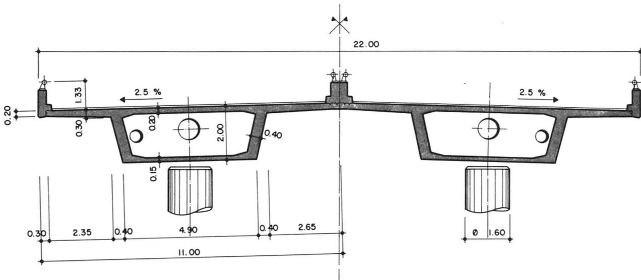
At its widest point, the cross-section of the superstructure is transformed into a multi-cellular hollow section with the addition of 2 webs and by closing the bottom slab over the whole width. Of course, the outer profile of the consoles is maintained. The continuation of the webs coming from the standard section had to be maintained in a skew position inside the multi-cell section for constructional reasons.
