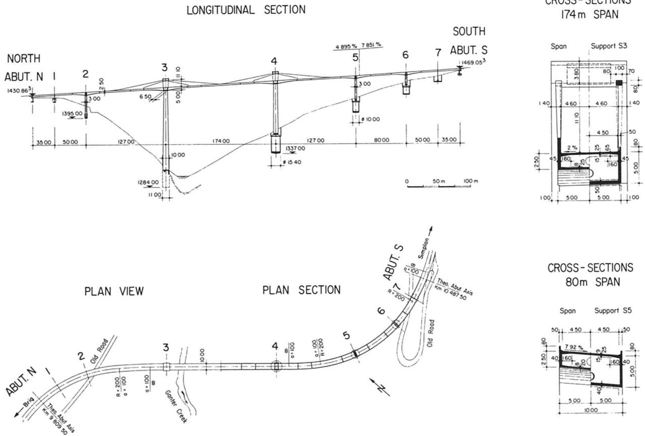
Fig. 2 Plan and Sections of the Bridge
