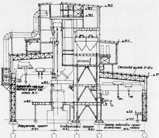
Fig. 1 Cross Section of the Shop with 400 ton Capacity Converters
