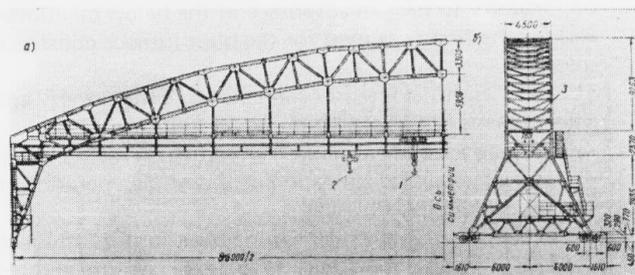
Fig. 2 Gantry Crane Made of Aluminium Alloys
