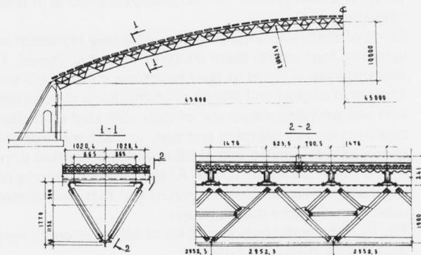
Fig. 1 Trusses for the Laboratory Building Roof
