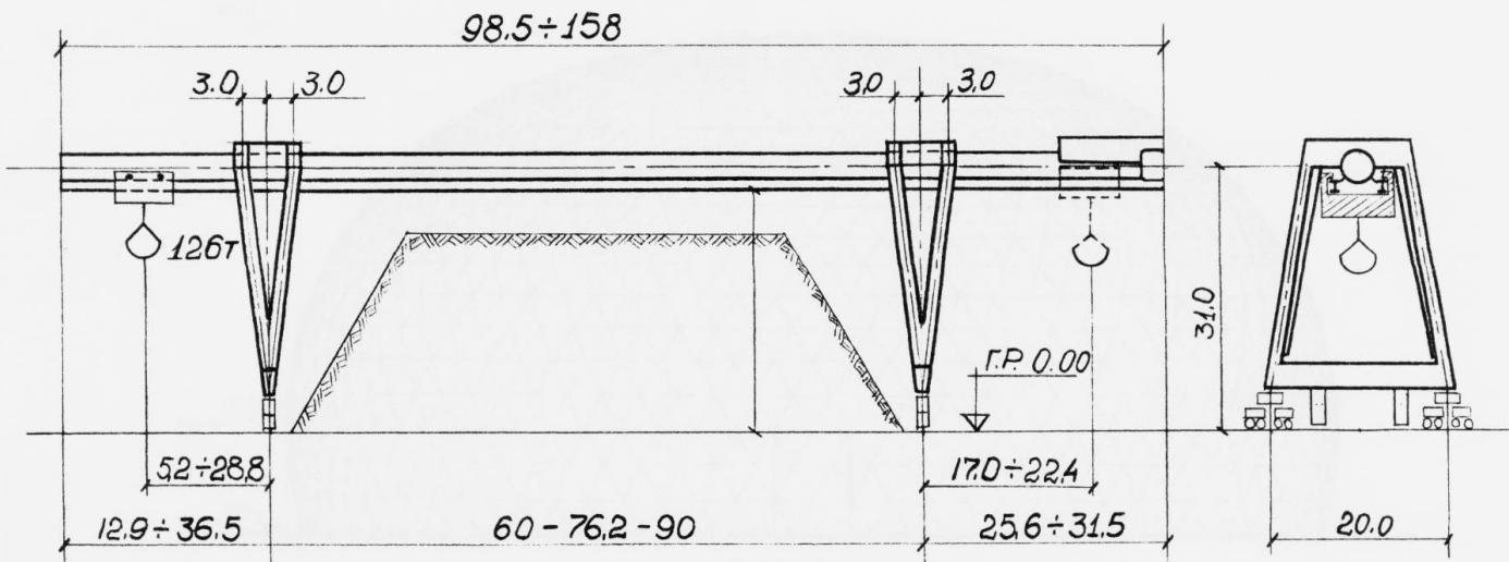
Fig. 1 A Loading Crane of a Pipe-girder Type
