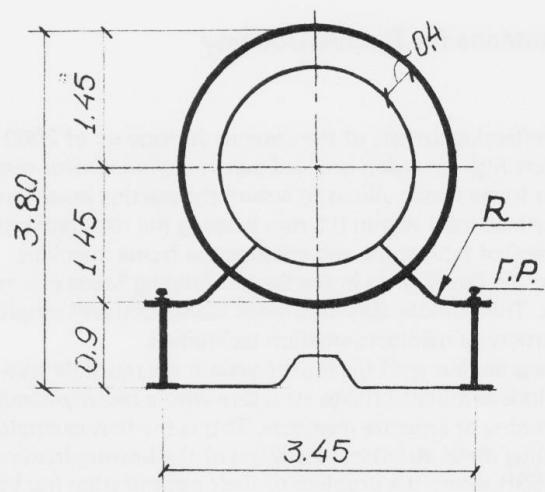
Fig. 2 Cross-sectional View of the Bridge
