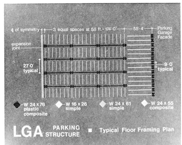
The building was divided into four approximately equal areas by means of expansion joints. A bracing system using stairwells as shear walls was designed to resist all lateral forces including wind, temperature and loads caused by lateral displacement. This system made it possible to relieve the steel frame of all horizontal forces.
