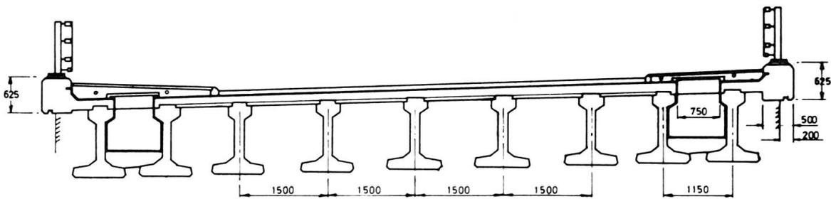
Fig 3 M-beams with composite in-situ slab
