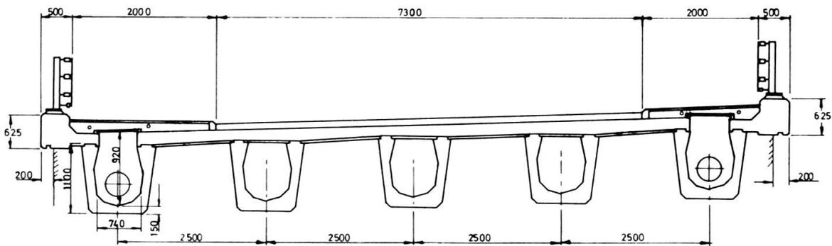
Fig 4 P.C. U-beams with in-situ composite slab
