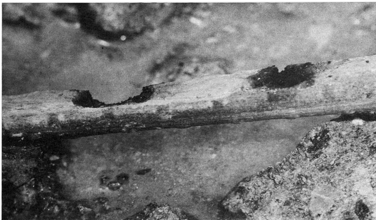
Localised corrosion on steel in concrete
