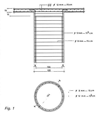
The function of the pipes underneath the slab is not to support the slab as is the case with a pit foundation, but to maintain the slab stiff and flat because these pipes do not reach hard layer under the slab to stand on, but on the other hand they «hang» on the slab.
