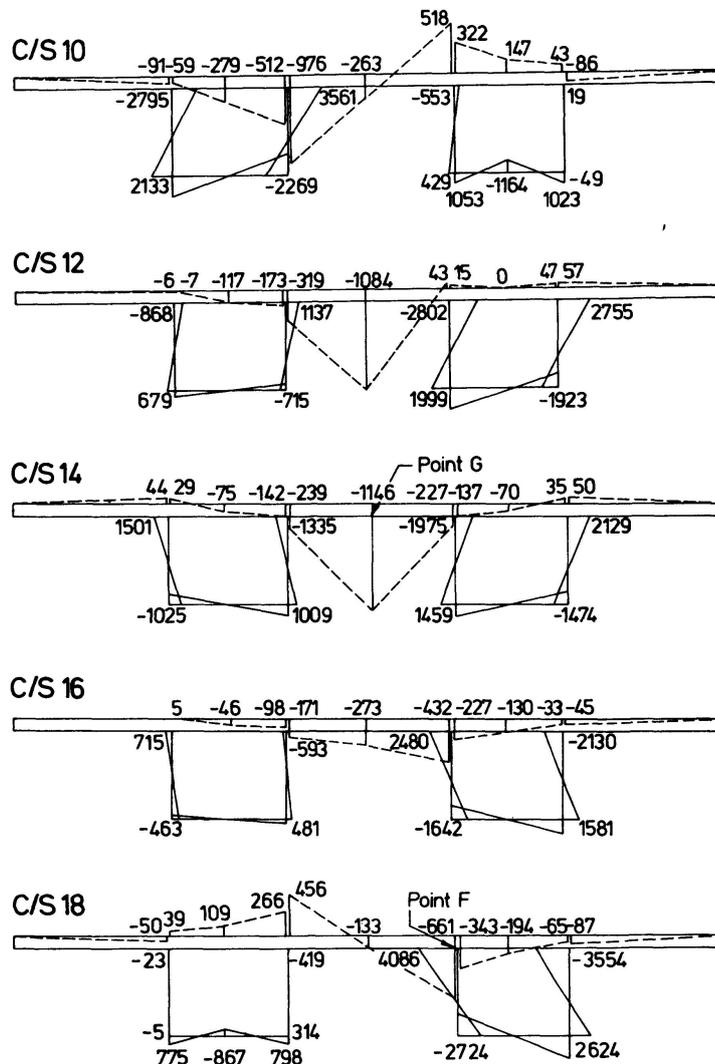
Fig. 13. Finite Element transverse Stresses for Load Case 3.
