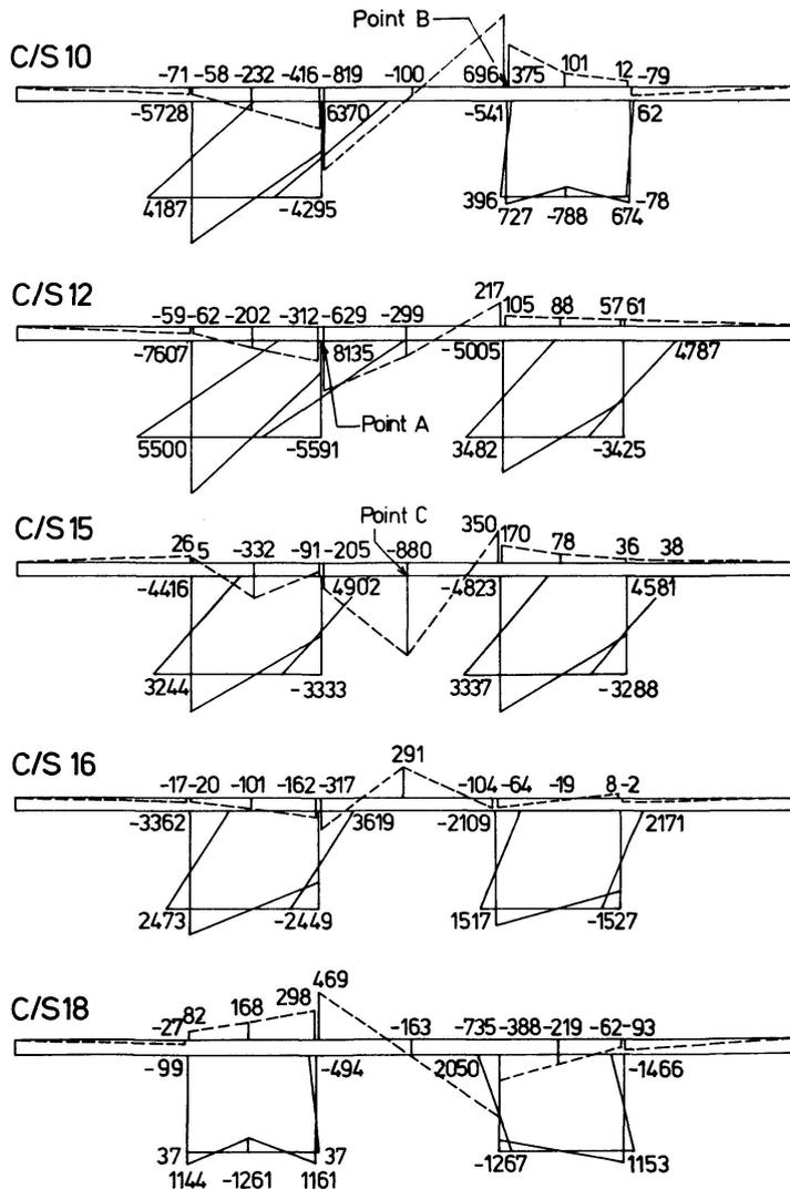
Fig. 11. Finite Element Transverse Stresses for Load Case 1.
