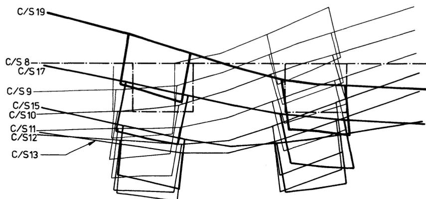
Fig. 10. Finite Element Deflections for Load Case 3.
