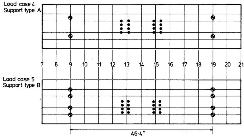
Fig. 15. Equivalent right Bridge Structures showing loading Positions 4 and 5 and alternative Support Arrangements. The section numbers have been chosen to coincide as far as possible with those of the skew structure.
