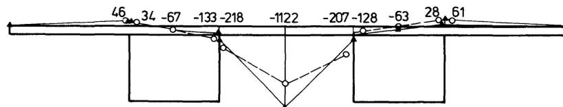
Fig. 7c. Transverse Stresses at Section 14 for Load Case 3.
