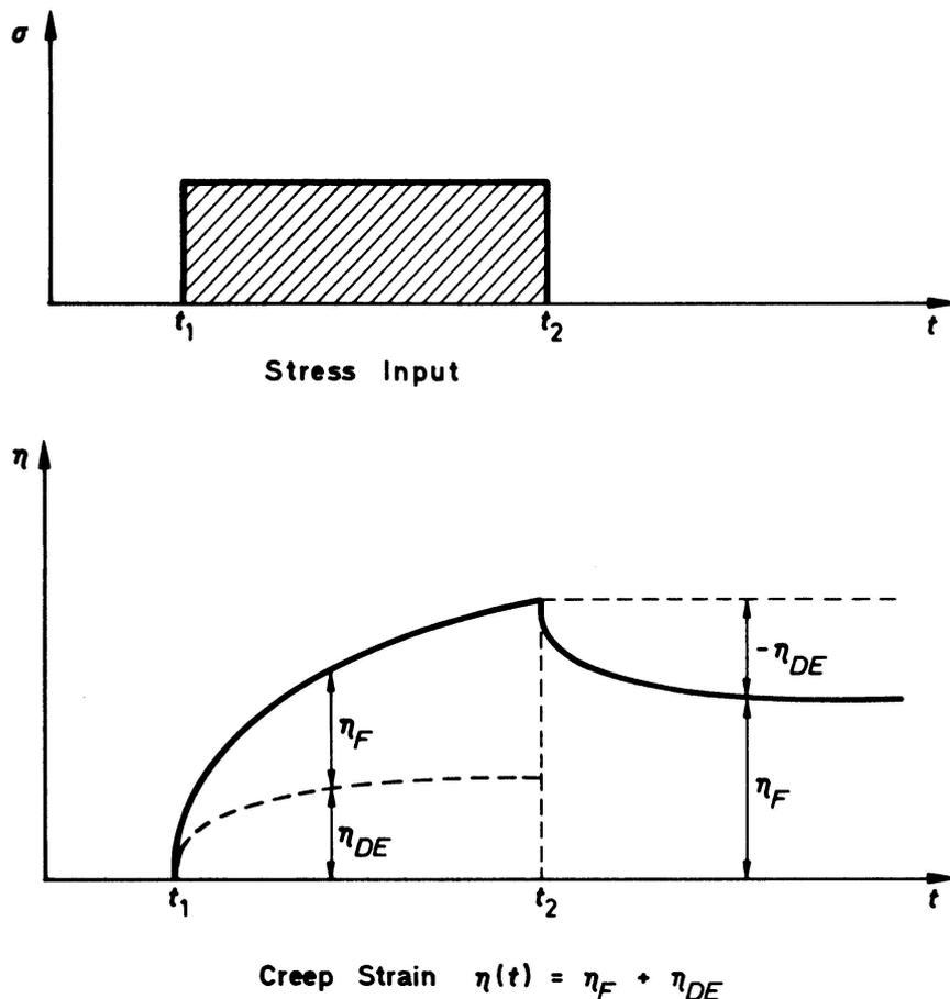
Fig. 2. Recoverable-Irrecoverable Creep Deformations.
