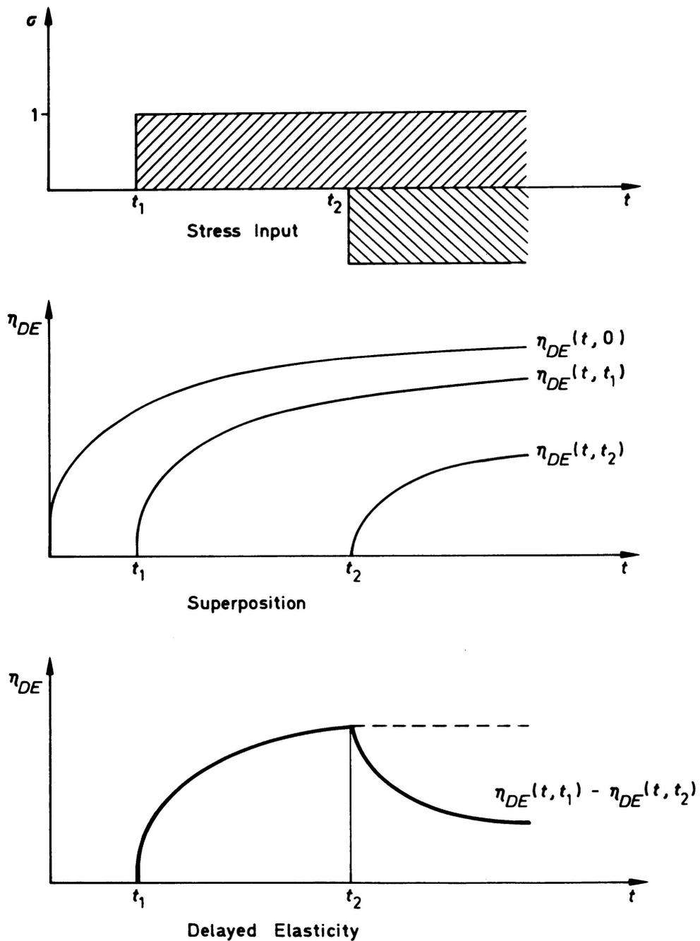
Fig. 6. Delayed Elastic Model (Mc Henry Superposition).
