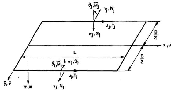
Fig. 5. Displacement Component in Local coordinate System.
