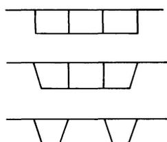
Fig. 1. Typical Box Girder Bridge Cross Section.
