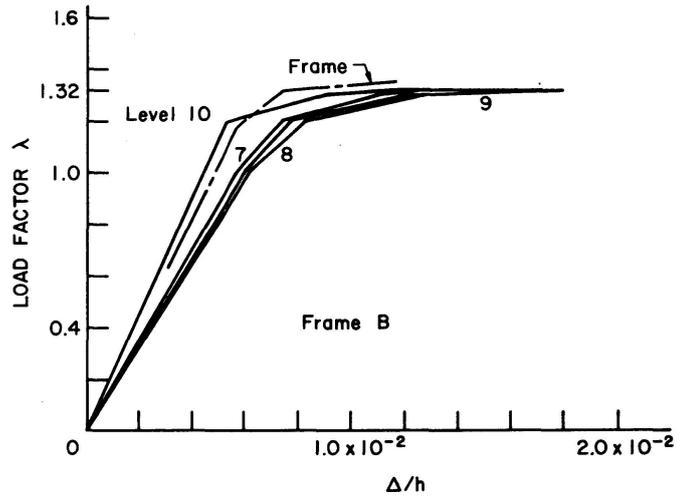
Fig. 9. Load-Deformation Curves of Frame B Stories.
