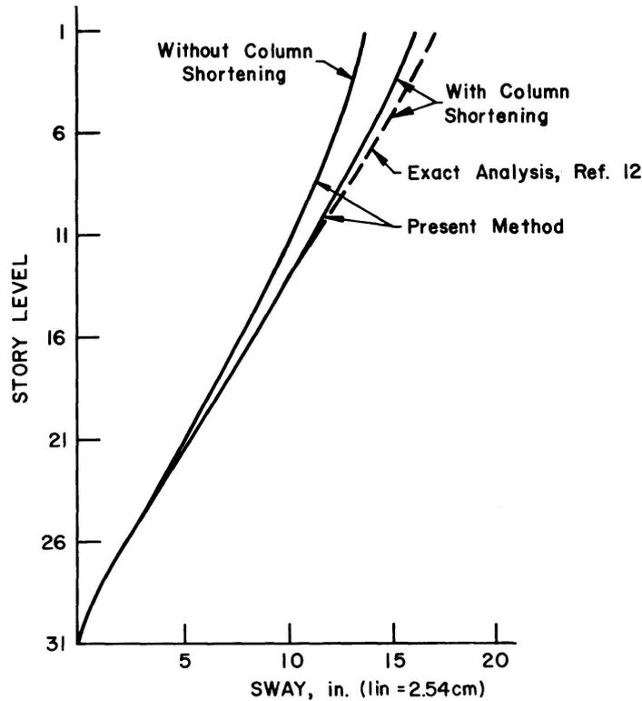
Fig. 5. Load-deformation Relationship of Frame a at  $\lambda = 1.0$ .
