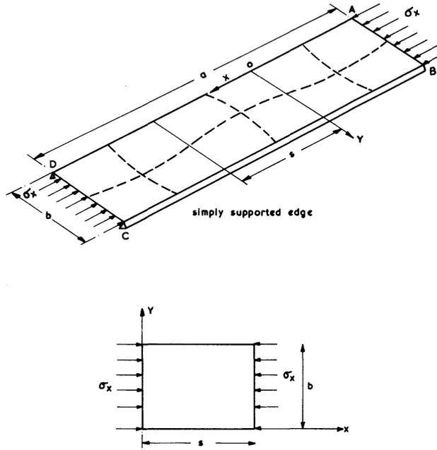
Fig. 1. Axial Loading on a simply supported Plate.
