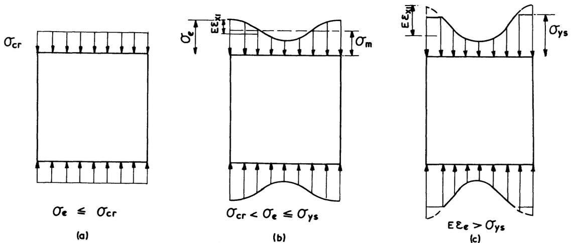
Fig. 2. Stress Distribution on a straight compressed Plate.
