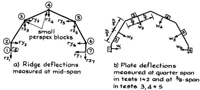
Fig. 8. Positions of Deflection Measurements during Tests.
