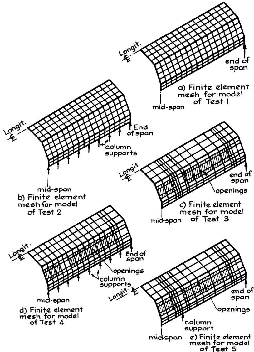
Fig. 10. Illustration of Meshes used in the Finite Element Solutions.
