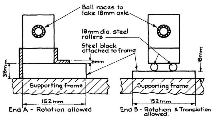
Fig. 7. Side View of End Support Assemblies.
