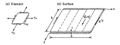
Fig. A-1. Membrane deck action.
