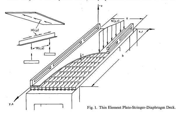
components have negligible out-of-plane stiffness and 2) are simply supported at the ends. Thus, the linear superposition of several solutions is required to analyze decks that are continuous over intermediate supports.
