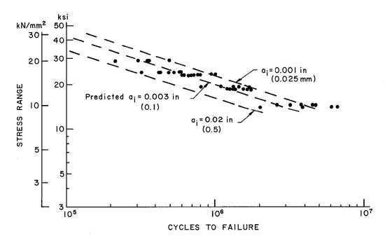
Fig. 18. Comparison of Predicted Fatigue Life with Test Data for Stiffeners Welded to Web and Flange.
