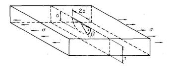
Fig. 12a. Part-through Crack in a Flat Plate.
