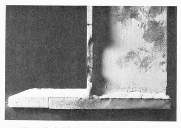
Fig. 6. Typical Fatigue Crack Surface at Failure.
