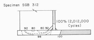
Fig. 3. Stages of Crack Growth at Stiffener-to-Flange Connection.
