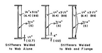
Fig. 1. Details of Test Girders.
