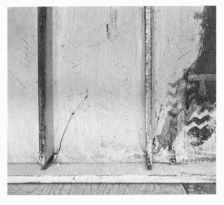
Fig. 7. Typical Failure at Web Stiffeners.
