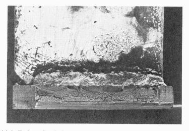
Fig. 5. Multiple Fatigue Crack Growth at the Toe of Stiffener-to-Tension Flange Weld.
