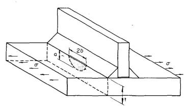
Fig. 12b. Part-through Crack at the Toe of a Non-load Carrying Fillet Weld.
