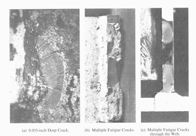
Fig. 9. Fatigue Crack Growth at the Toe of Stiffener-to-Web Weld.
