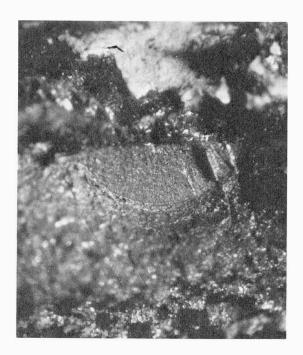
Fig. 4. 0.028-inch Deep Crack at the Toe of the Stiffener-to-Tension Flange Weld.
