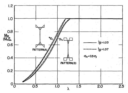
Fig. 5. Comparison between residual stress patterns.
