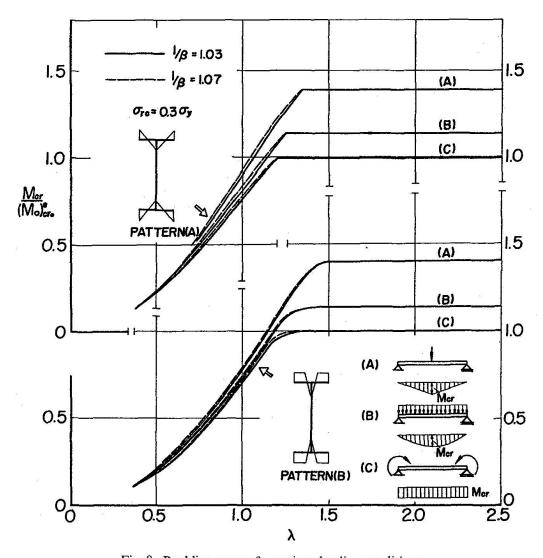
Fig. 8. Buckling curves for various loading conditions.
