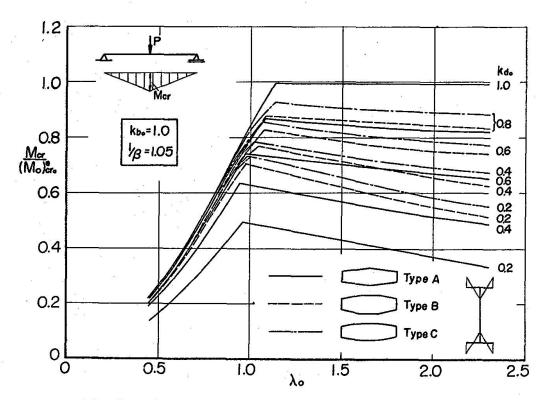
Fig. 10. Buckling curves of plate girders with tapering web depths.
