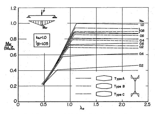
Fig. 9. Buckling curves of plate girders with tapering flange widths.
