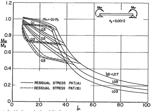
Fig. 3. Effect of residual stress levels and distributions. **b**
