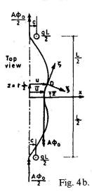
application of the uniform load q moves horizontally an amount  $u + \phi d$  and lowers a little more than 0 (Fig. 4a). Each end support again provides a torsional couple  $\frac{A\phi_0}{2}$ , but, besides, a couple of magnitude  $c \cdot \frac{qL}{2} = q \int_0^{L/2} (u + \phi d) dz$  necessary to offset the horizontal deviation of the load q.
