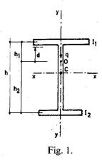
3) Owing to symmetry, buckling does not change the direction of the flanges at mid-span:
