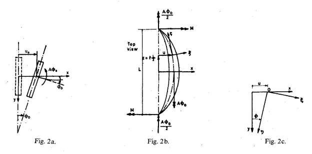
The differential equations for horizontal bending and for twisting of the beam, as written by Timoshenko [3] and taking account of the moment  $\frac{A\phi_0}{2}$ , are, for the half-beam with positive coordinates z:
