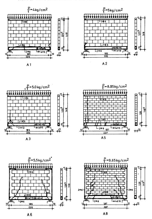
Fig. 3. Series A, Specimens and Modes of Failure.
