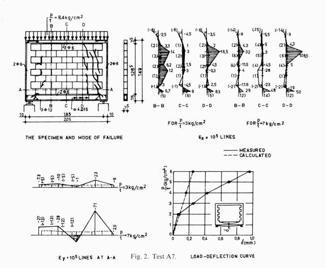
Fig. 3 shows the crack patterns at ultimate load and in Fig. 4 the curves of mid span deflection of bottom beams.
