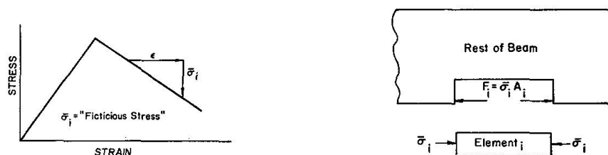
Fig. 6. Fictitious stresses and forces.
