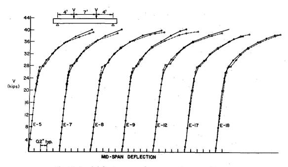
Fig. 10. Load-deflection curves for prestressed concrete I-beams.
