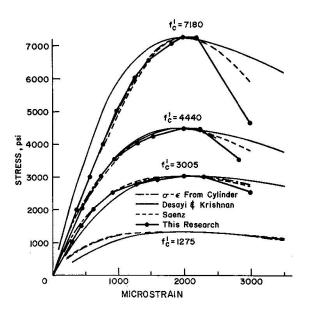
Fig. 3. Comparisons of concrete stress-strain curves.
