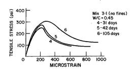
Fig. 4. Concrete tensile stress-strain curves.
