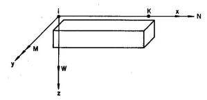
Fig. 1. Coordinate system and positive sign convention.
