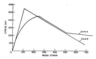
Fig. 5. Analytic tensile stress-strain curves.
