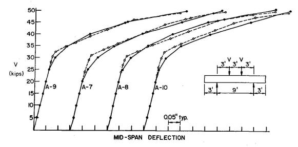
Fig. 9. Load-deflection-curves for prestressed concrete solid box beams.
