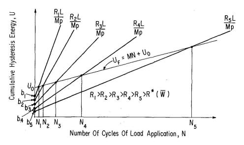
Fig. 12. Cumulative hysteresis energy versus number of cycles of load application.
