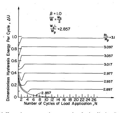
Fig. 6. Hysteresis energy per cycle versus number of cycles of load application.
