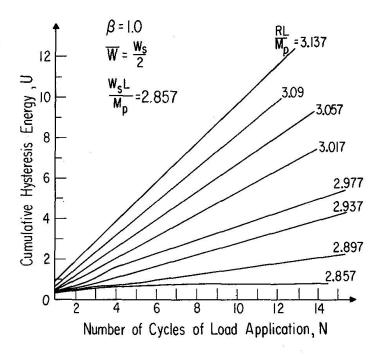
Fig. 11. Cumulative hysteresis energy versus number of cycles of load application.
