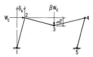
Fig. 4. Collapse mechanism.
