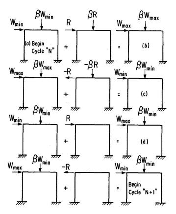
Fig. 5. The  $N^{th}$  cycle of load applications.
