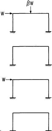
Fig. 3. One cycle of load applications.
