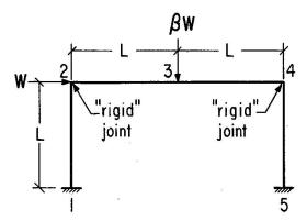
Fig. 1. Three-bar hyperstatic portal frame.
