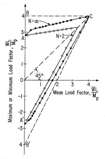
Fig. 10. Load factor versus mean load factor diagrams,  $\beta = 0.5.\,$
