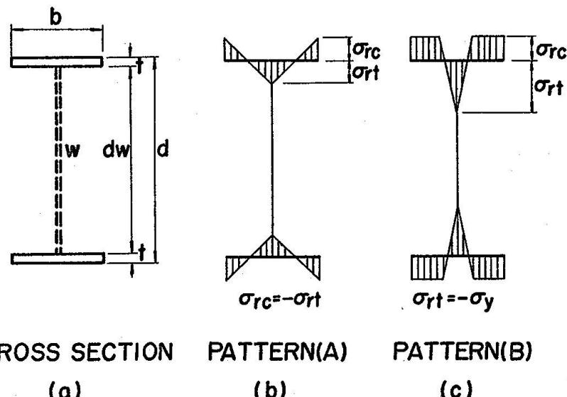
Fig. 1. Simplified cross section and idealized residual stresses.
