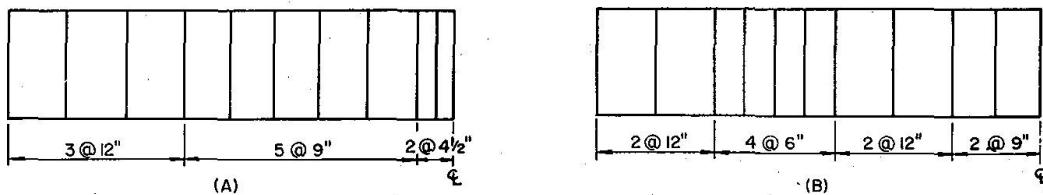
Fig. 8. Elemental discretization.
