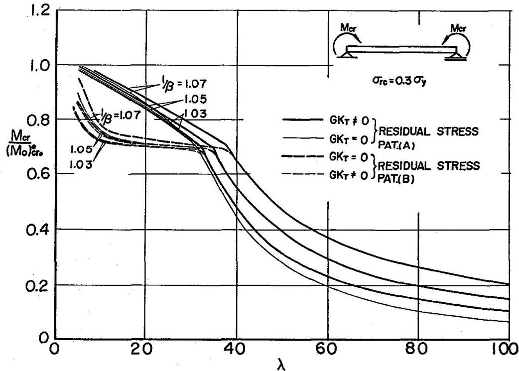
Fig. 6. Effect of St. Venant torsional stiffness.
