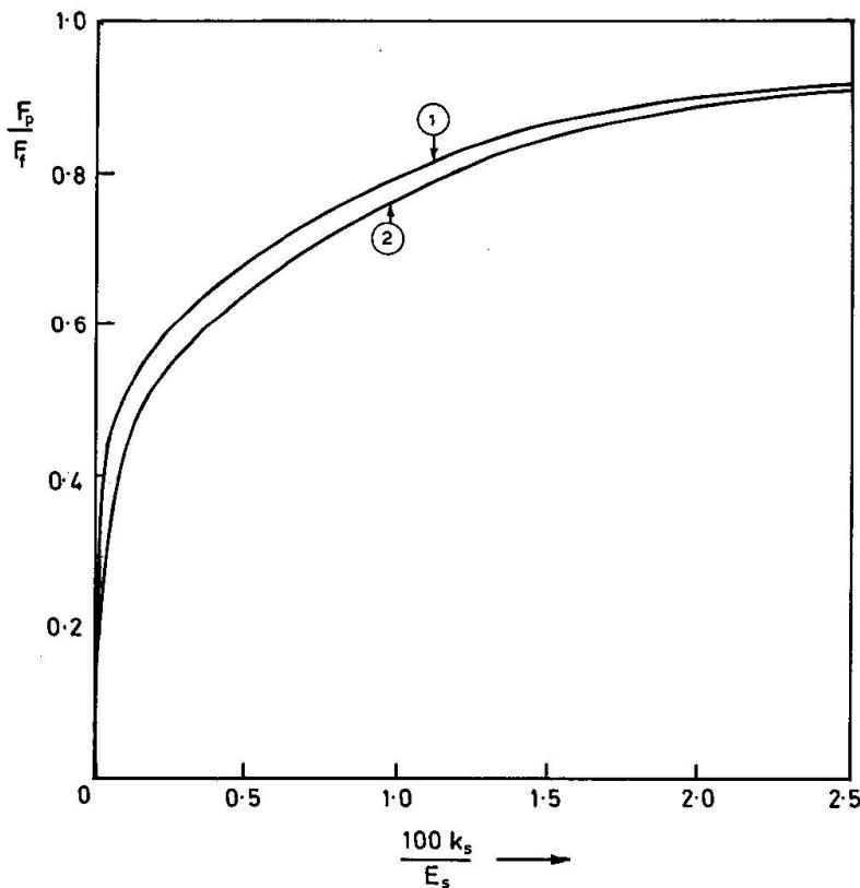
Fig. 3. Degree of interaction against foundation modulus.
