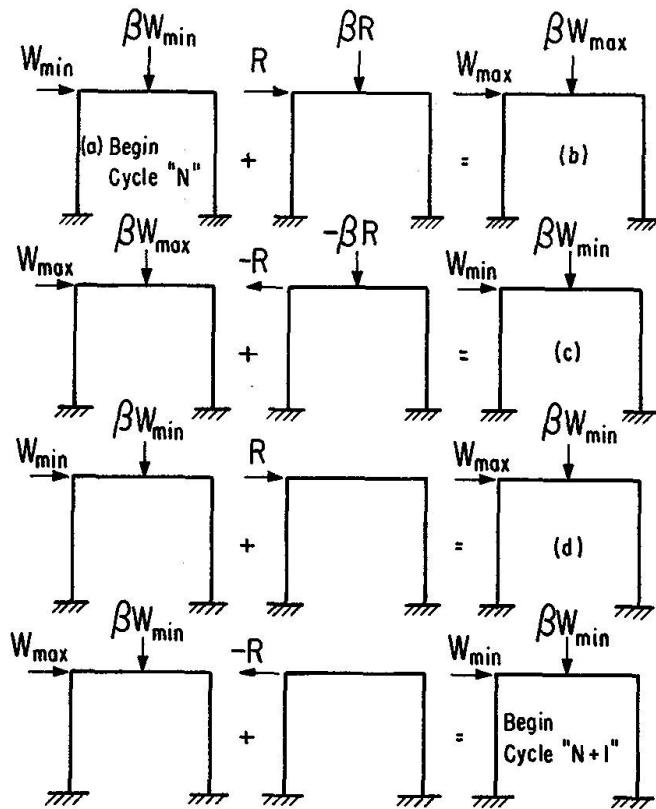
Fig. 5. The  $N^{\text{th}}$  cycle of load applications.
