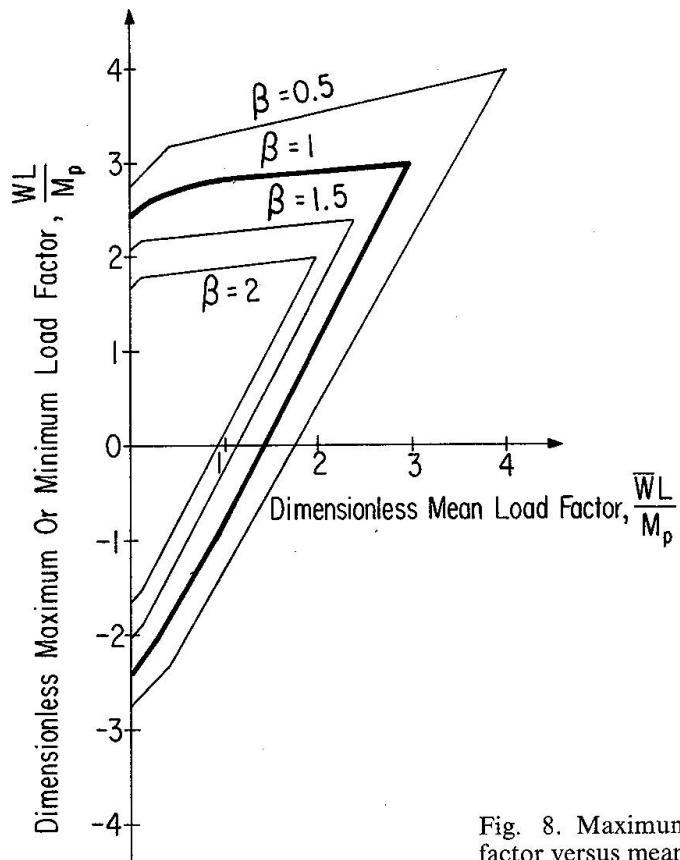
Fig. 8. Maximum or minimum load factor versus mean load factor diagrams.
