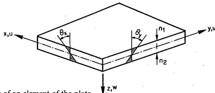
Fig. 1. Deformations of an element of the plate.
