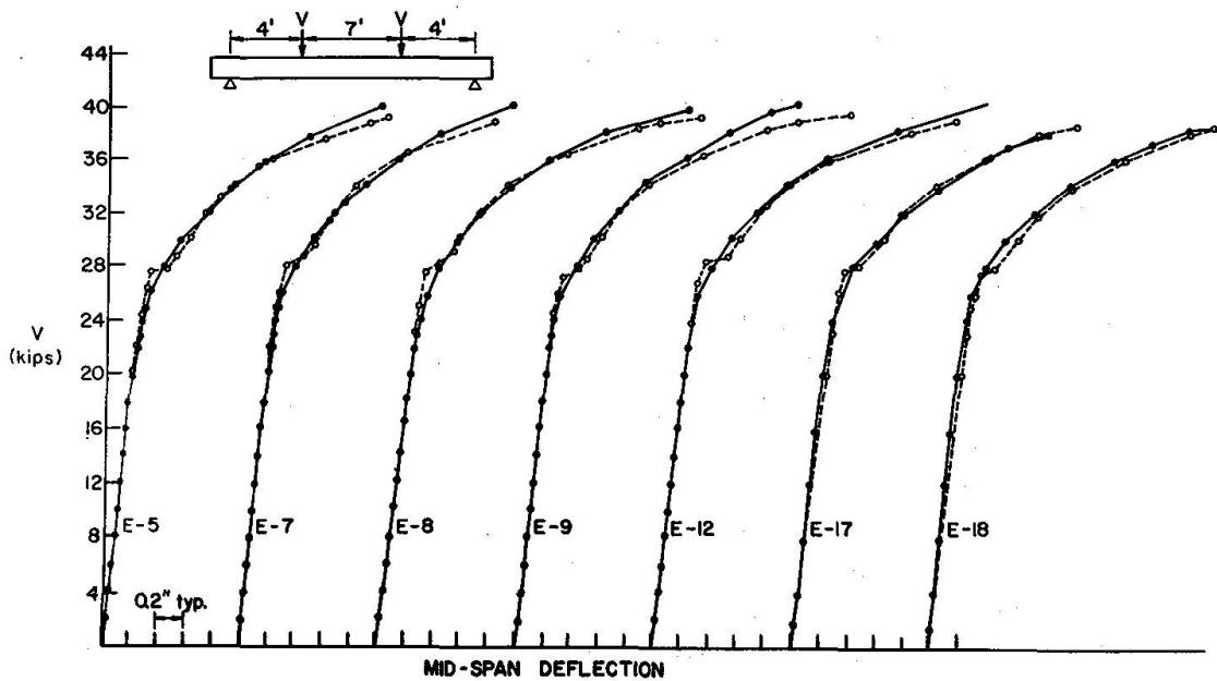
Fig. 10. Load-deflection curves for prestressed concrete I-beams.
