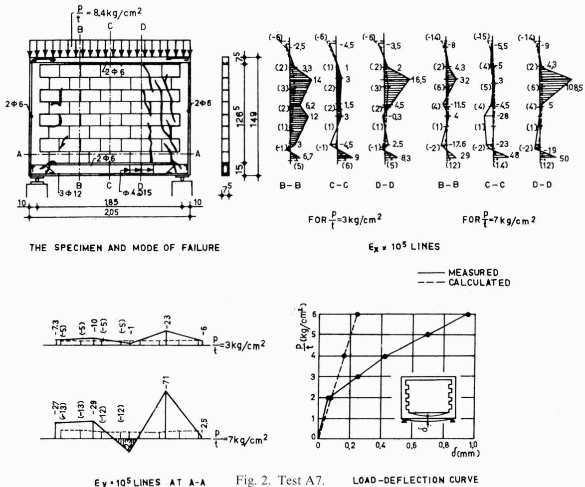
Fig. 2. Test A7. LOAD-DEFLECTION CURVE
