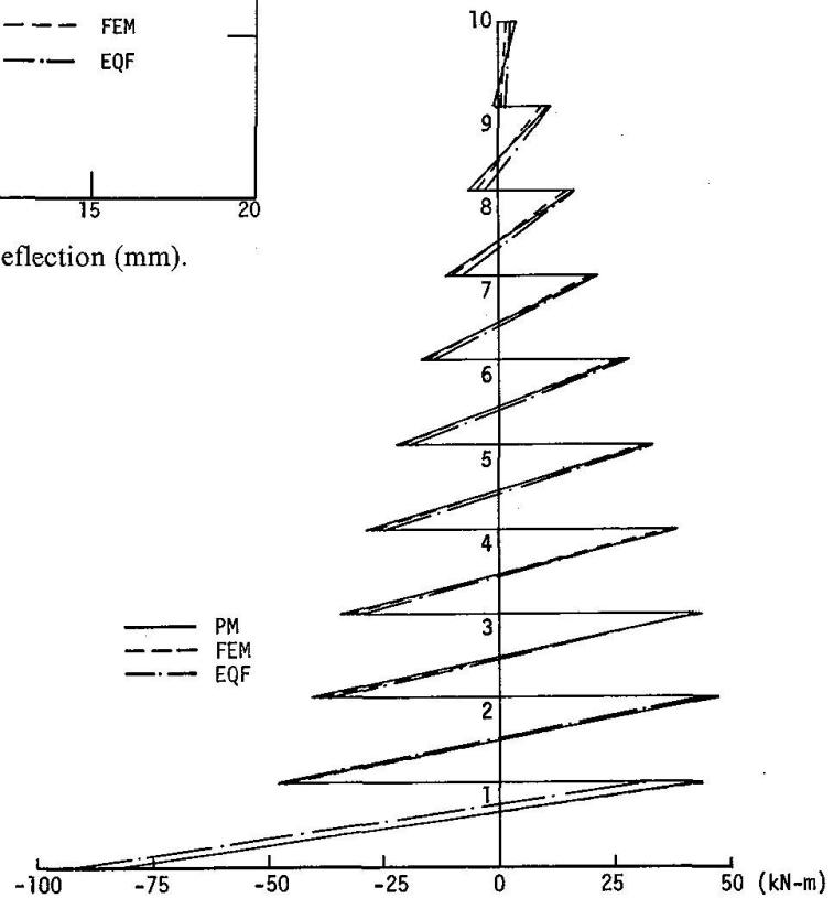
Fig. 7. Example 1: bending moment diagram of exterior column.
