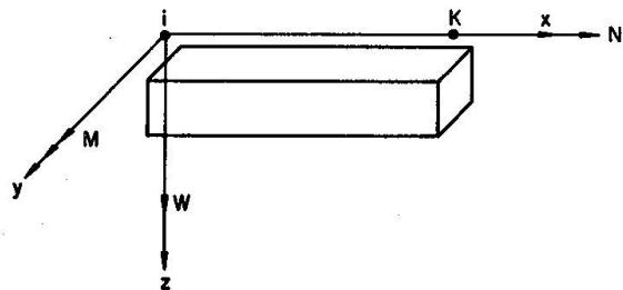
Fig. 1. Coordinate system and positive sign convention.
