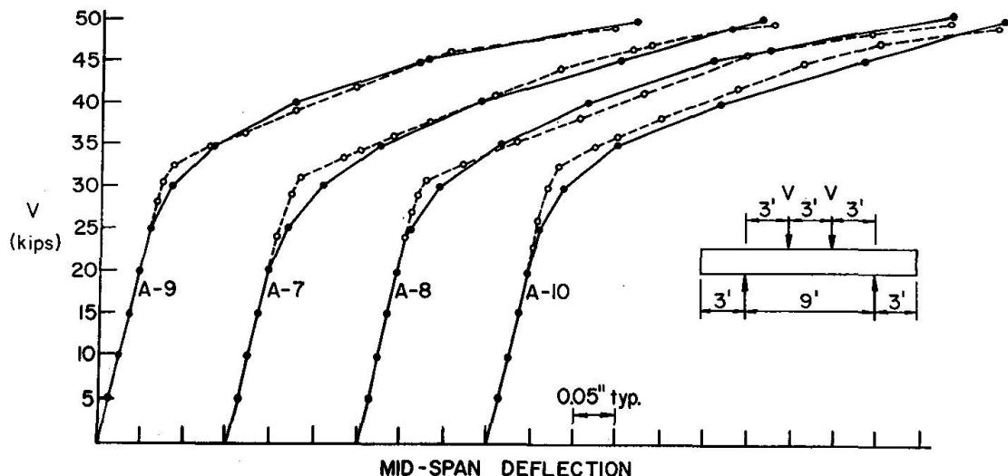
Fig. 9. Load-deflection-curves for prestressed concrete solid box beams.
