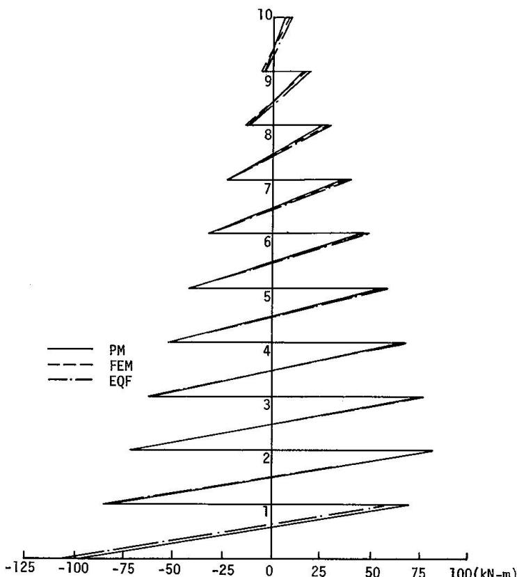
Fig. 8. Example 1:bending moment diagram of interior column.
