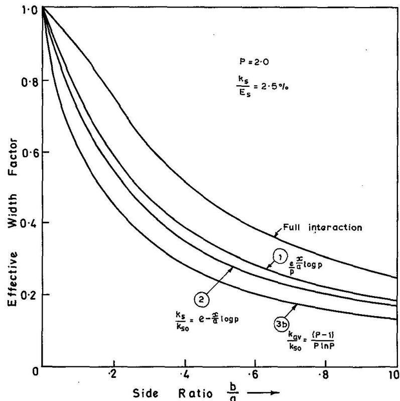
Fig. 5. Variation of Effective width with aspect ratio.
