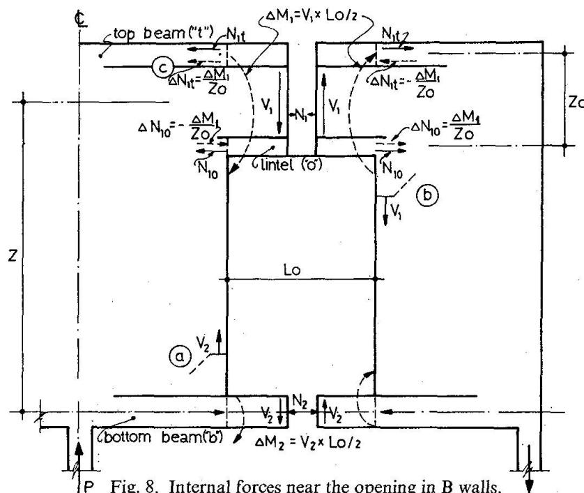
Fig. 8. Internal forces near the opening in B walls.
