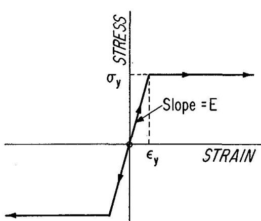
Fig. 2a. Stress Versus Strain.
