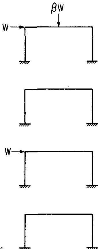
Fig. 3. One cycle of load applications.
