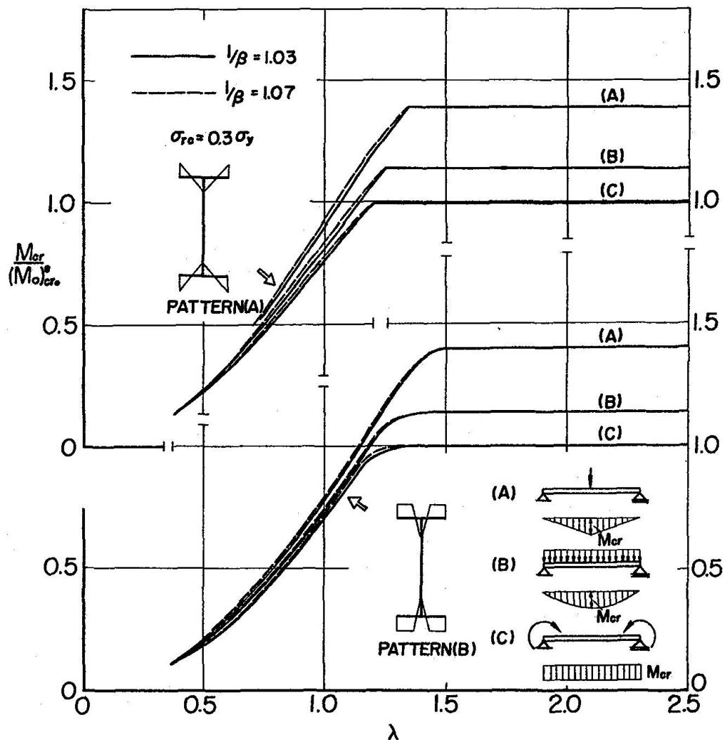
Fig. 8. Buckling curves for various loading conditions.
