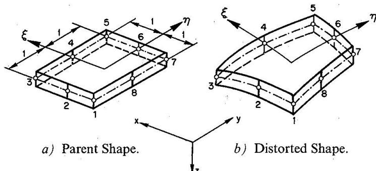
Fig. 2. The quadratic isoparametric plate bending element:
