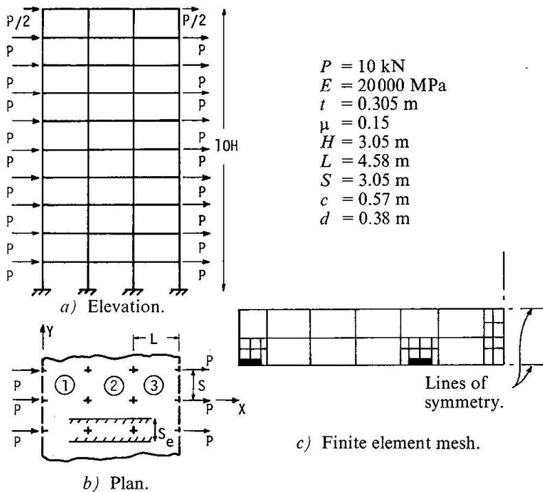
Fig. 4. Example 1: Interior bay of a 10 storey building.
