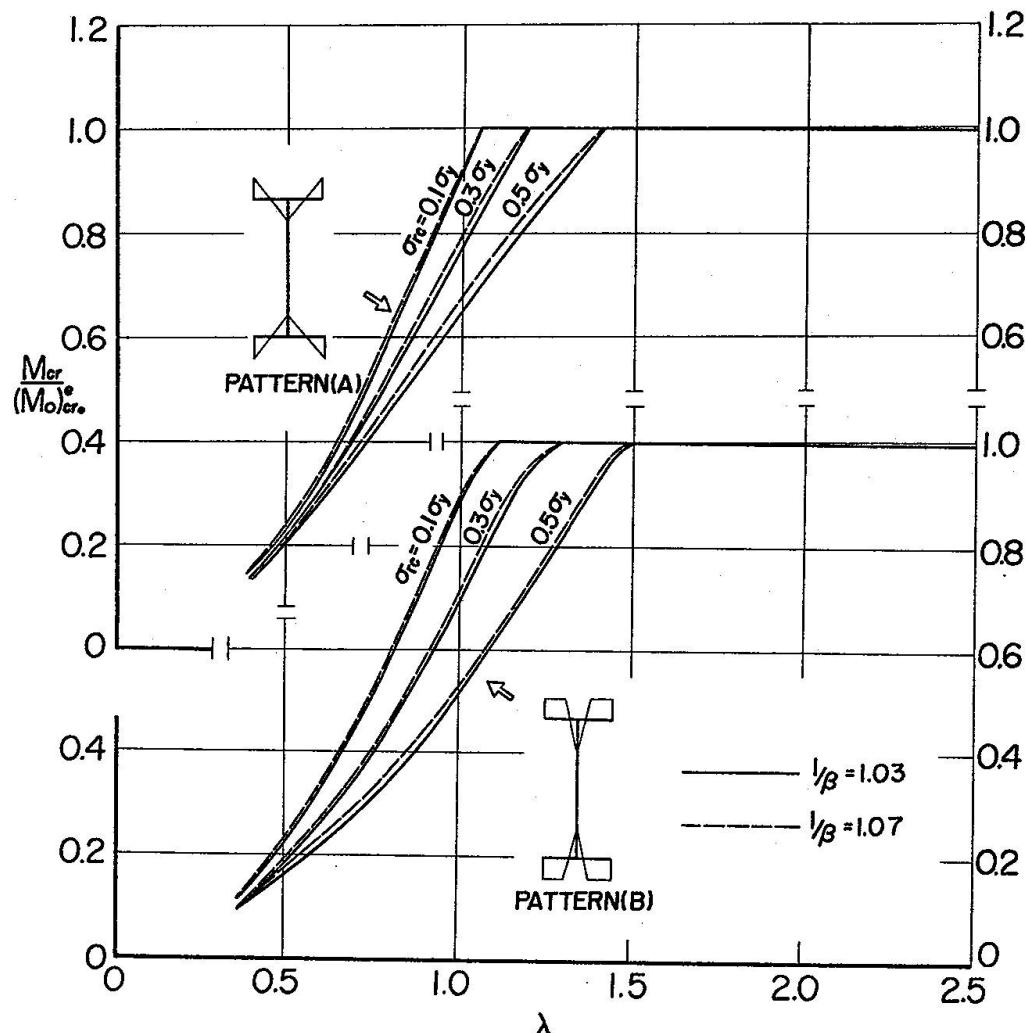
Fig. 4. A possible representation of buckling curves.
