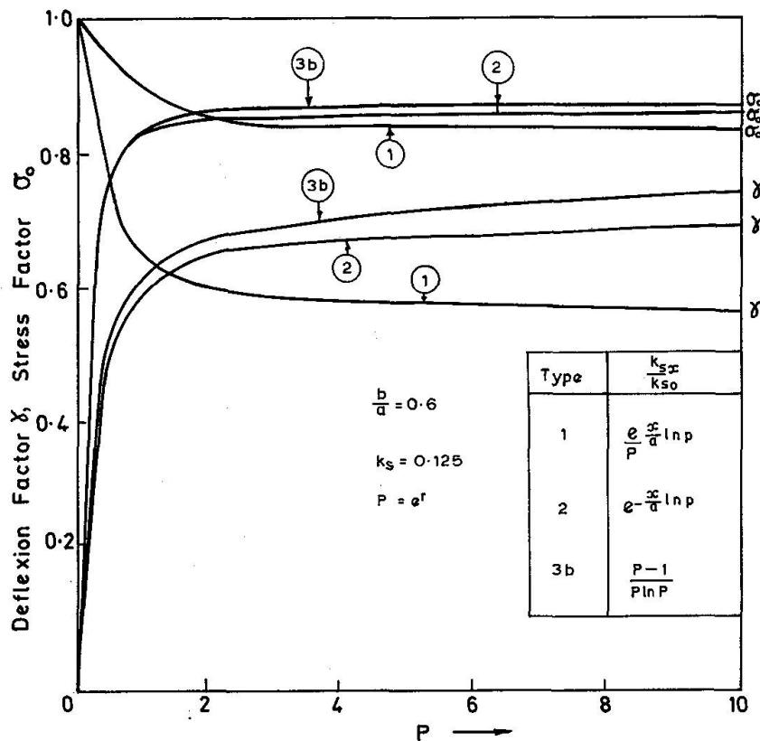
Fig. 2. The effect of foundation modulus reduction parameter  $p$  on deflections and stresses.
