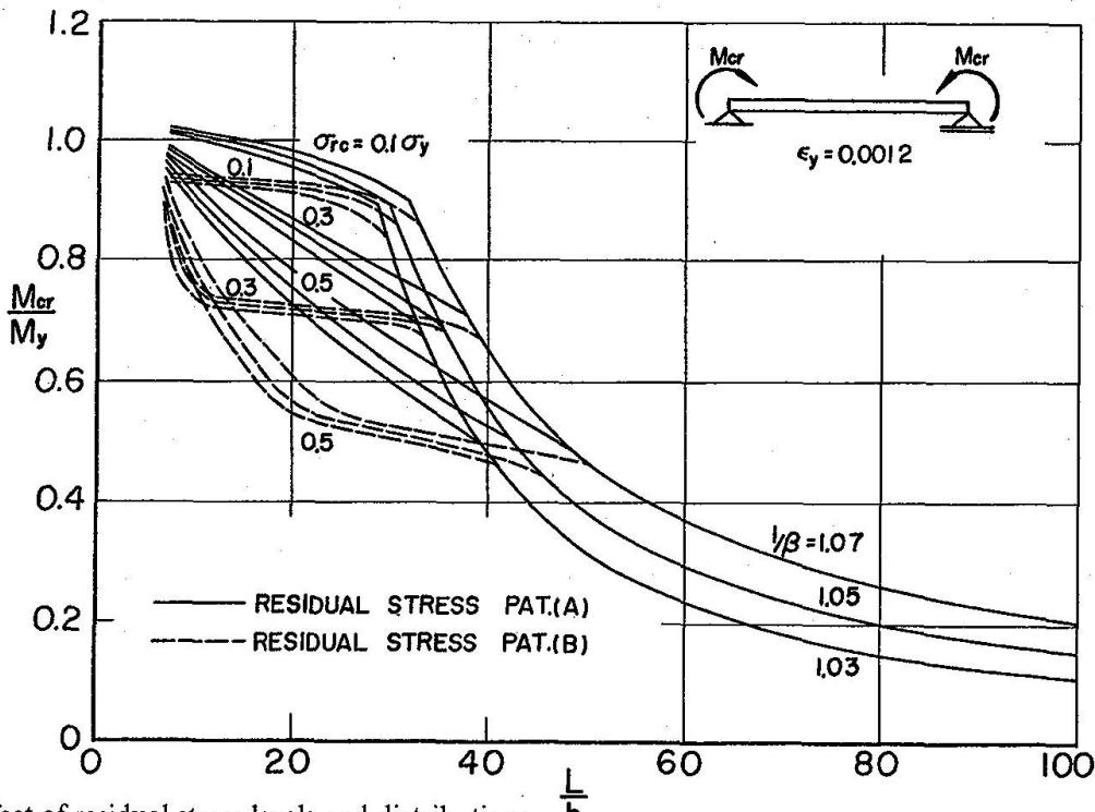
Fig. 3. Effect of residual stress levels and distributions.
