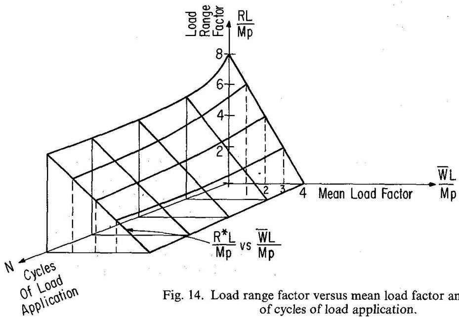
Fig. 14. Load range factor versus mean load factor and number of cycles of load application.
