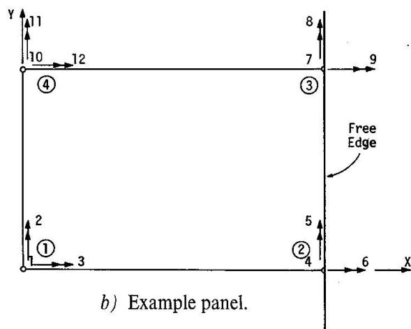
Fig. 10. Panel rotation to suit boundary conditions.
