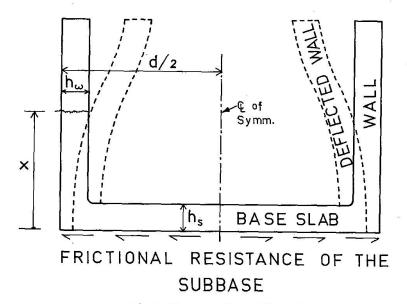
Fig. 2. Cross section of the tank.
