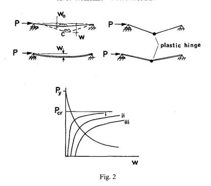
Fig. 2b, we determine the curve (iv) in Fig. 2c. This method assumes that there is a sudden transition from elastic to plastic mode at the intersection of the curves. Of course in reality there is a gradual spread of plasticity across the section, but because most of the energy in the column in both the elastic and plastic modes is bending strain energy this approach has in the past been a sufficiently accurate and useful aid in describing the behaviour of struts and frameworks [10].
