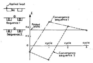
Fig. 12b. Illustration of convergence of solution for discreet cell girder.
