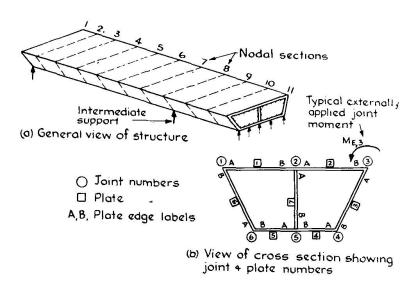
Fig. 4. Typical structure considered in the analysis.
