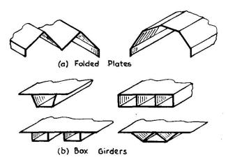
Fig. 1. Typical folded plate and box girder cross-sections.
