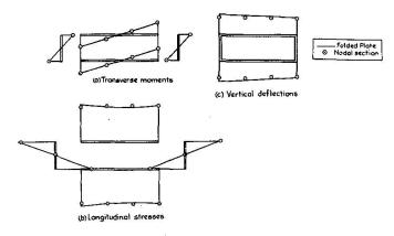
Fig. 17. Distribution around midspan cross-section of typical girder.
