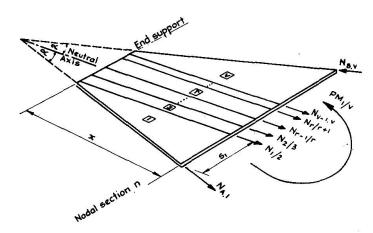
Fig. 8. Forces set up in a typical plate beam unit containing several co-planar plates.
