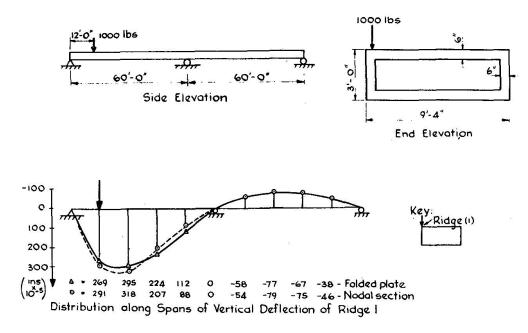
Fig. 20. Results for unsymmetrically loaded continuous girder.
