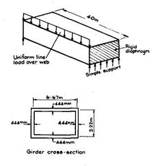
Fig. 13. Details of typical single-cell girder.
