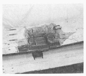
Fig. 9. Concrete removed at failure location in MS3.
