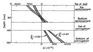
(a) Strain distributions during fatigue tests
