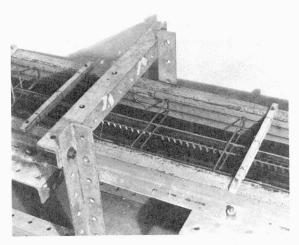
Fig. 2. Specimen DS3 before casting.
