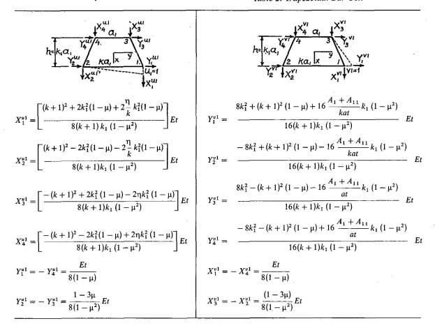
The nodal forces of the flexural Condition 5 may be correlated with those of Condition 2 by observing the displacements of the joints and the action of the bars forming the cell (Fig. 9). Since both Conditions 2 and 5 are symmetrical about the vertical axis, the bars  $A_5$  and  $A_6$  are inactive.
