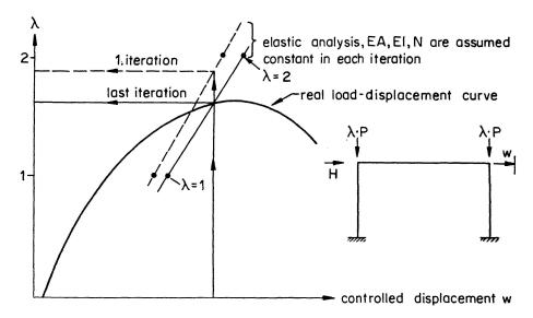
Fig. 13. Displacement controlled determination of a point on the real load-displacement curve.
