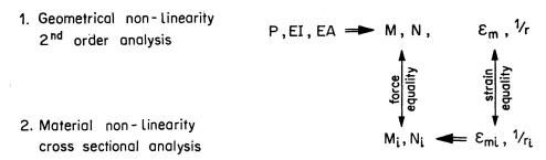
Fig. 1. Schematic illustration of the analysis.
