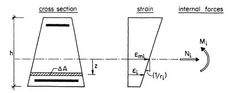
Fig. 7. Cross section, strain distribution and forces.
