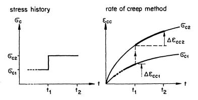
Fig. 9. Creep under variable stresses.
