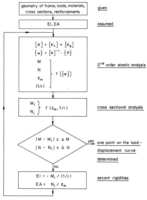
Fig. 11. Flow-chart for frame analysis.
