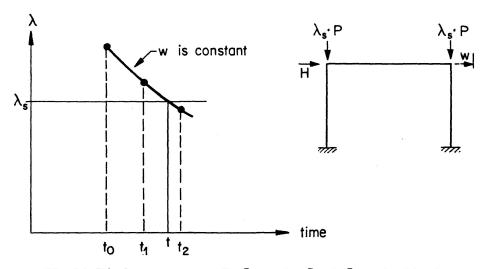
Fig. 14. Displacement controlled procedure under sustained loads.
