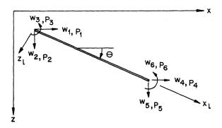
Fig. 4. Global forces and displacements.
