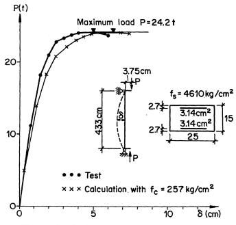
Fig. 15. Load-displacement curve (column 24).
