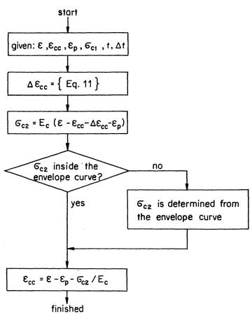
Fig. 10. Determination of stress and "plastic" strain.
