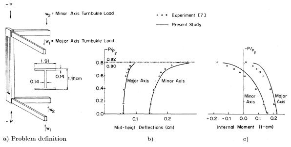
Fig. 6. Example 1: Rotationally restrained beam-column [7].
