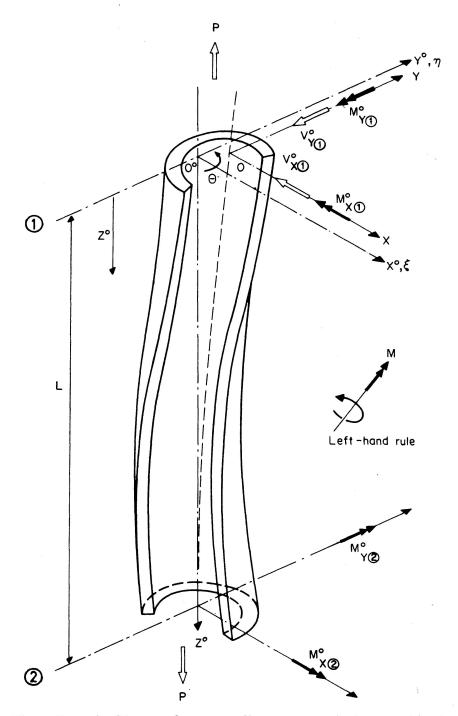
Fig. 1. Restrained beam-column, coordinate systems and external loads.
