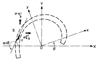
d) Shear stresses and projection of normal stresses in the section  $Z^0$  Fig. 10. Forces acting on an elementary area.
