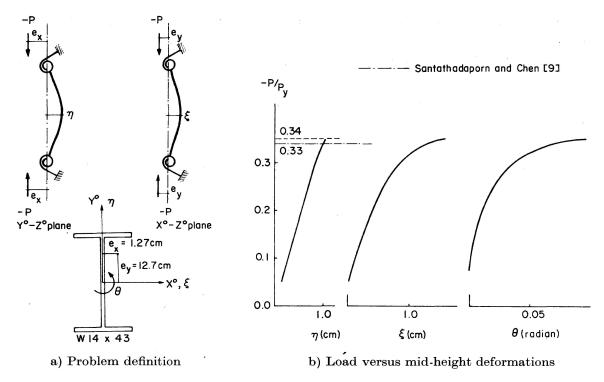
Fig. 7. Example 2: Rotationally restrained beam-column [9].
