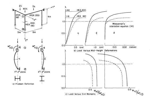
Fig. 9. Example 4: Three dimensional beam-column subassamblage.
