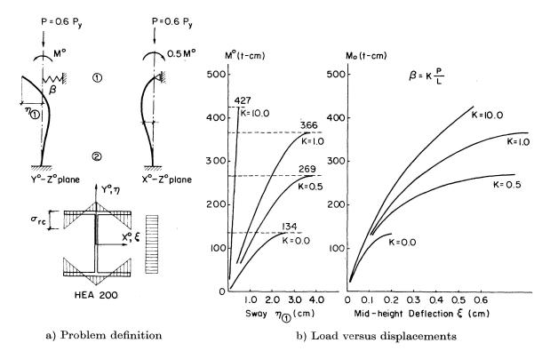
Fig. 8. Example 3: Directionally restrained beam-column.
