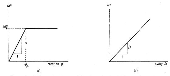
Fig. 4. Load-deformation characteristics of rotational and directional restraints.
