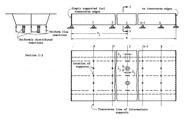
Fig. 1. Multi-cell box girder with intermediate supports.
