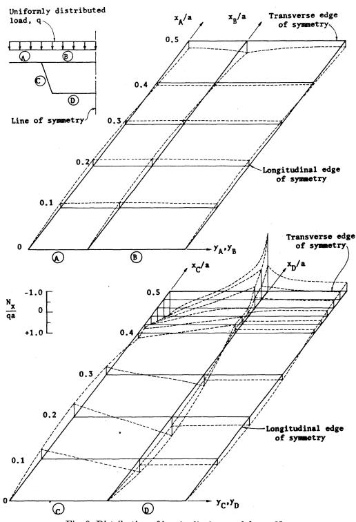
Fig. 9. Distribution of longitudinal normal force,  $N_x$ .
