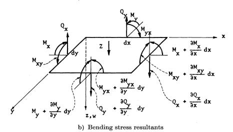
Fig. 2. Positive directions of stress resultants, displacement components and load components.
