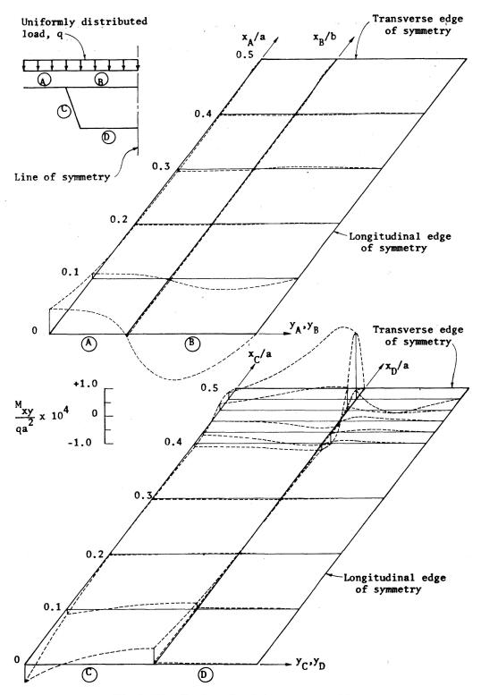
Fig. 7. Distribution of twisting moment,  $M_{xy}$ .
