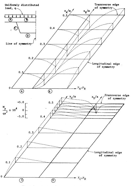
Fig. 5. Distribution of transverse bending moment,  $M_y$ .
