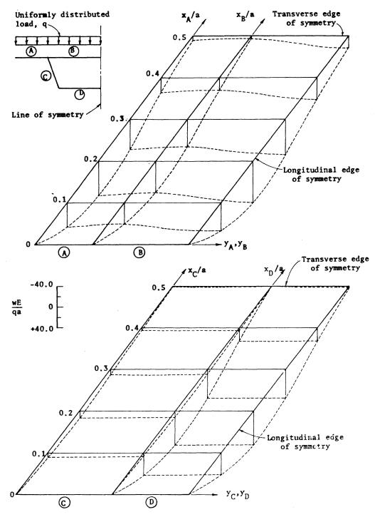
Fig. 4. Distribution of displacement component, w.
