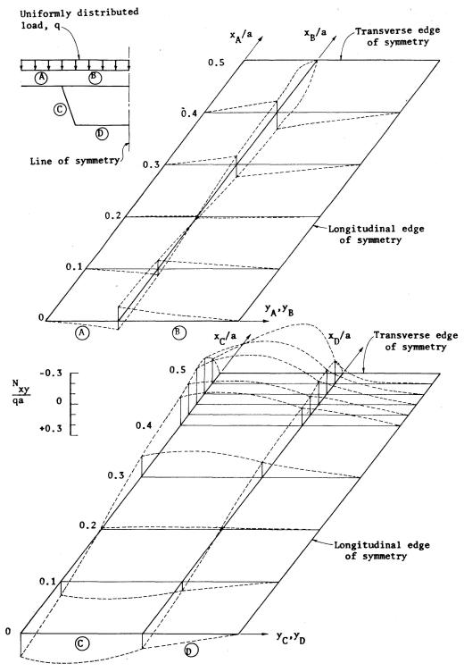
Fig. 10. Distribution of membrane shearing force,  $N_{xy}$ .
