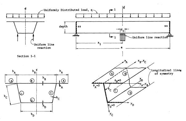
Fig. 3. Illustrative example - two-span single-cell box girder.
