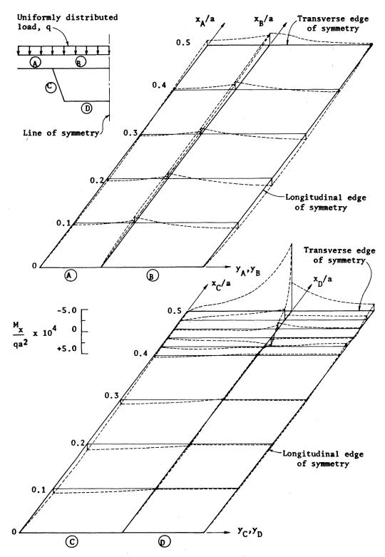
Fig. 6. Distribution of longitudinal bending moment,  $M_x$ .
