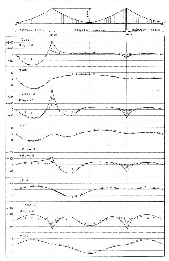
Fig. 4. Model of type 1 and test results.
