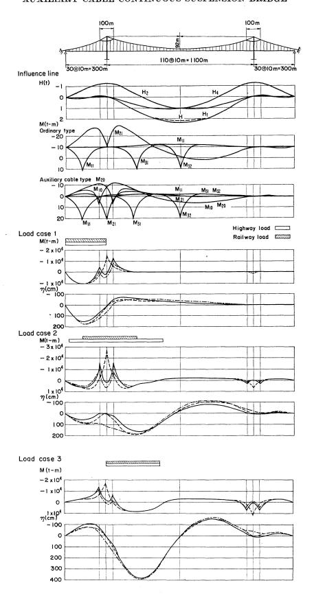
Fig. 11. Influence lines, bending moments and deflections of continuous suspension bridge.
