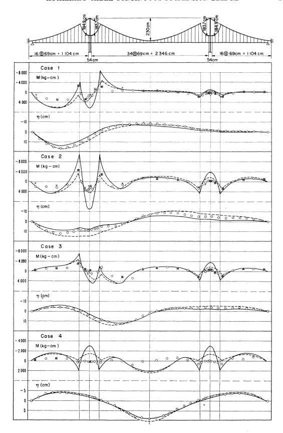
Fig. 6. Model of type 3 and test results.
