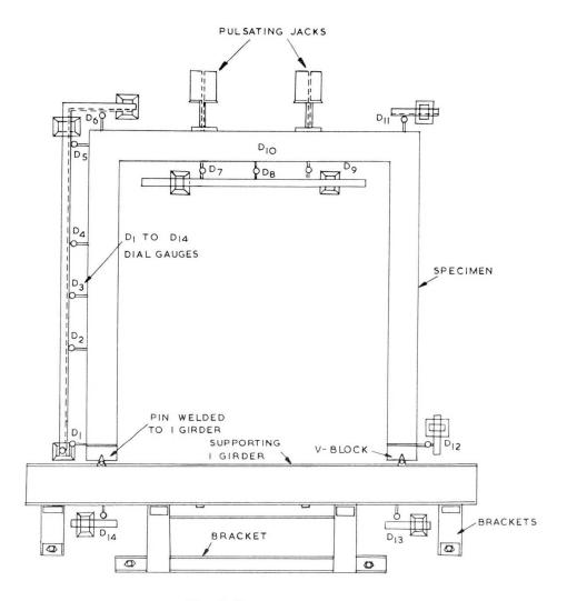
Fig. 2. Test setup.
