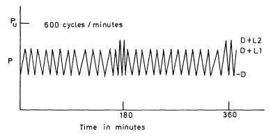
Fig. 5. Typical load cycle.
