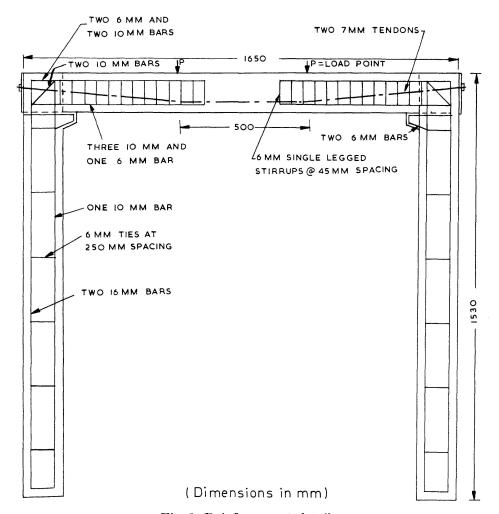
Fig. 1. Reinforcement details.
