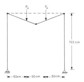
Fig. 4. Collapse mechanism.
