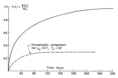
Fig. 4. Creep function used in calculations.
