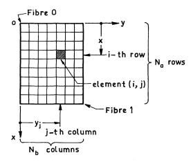
Fig. 2. Partitioning of concrete section.
