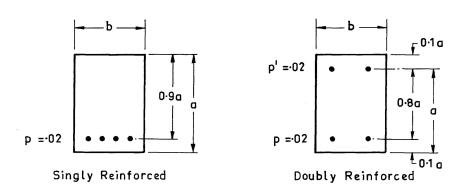
Fig. 7. Cross sections for numerical calculations.
