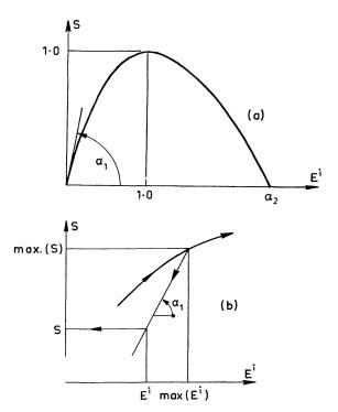
Fig. 3. Relation between stress and instantaneous strain.
