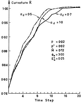
Fig. 14. Effect of parameter  $\alpha_d\text{-curvature.}$
